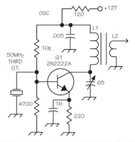
This is the *schematic* of the circuit represented by the box labeled "oscillator" in the block diagram of the crystal-controlled transmitter. The schematic shows individual electronic parts.
